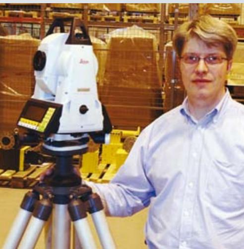
**Leading industrial robot manufacturer, ABB Robotics, in an industry first application, uses Leica's Laser Tracker Systems to guarantee movement precision during an innovative calibration process.**
