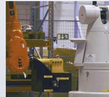
*Leica Laser Tracker can follow a movement of 6 m per second with an acceleration of 2G and measure 1,000 points per second. The accuracy of some 0.01 mm per metre suits ABB's work in supplying robots with lifelong position accuracy.*
