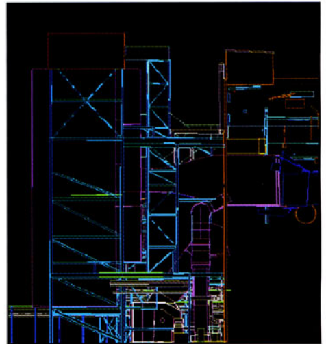
2D views can be extracted from the model data as necessary.
