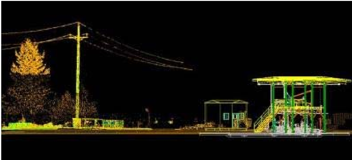
Image courtesy ProjEx Technologies Ltd. Captured MicroStation image shows referenced point cloud data with new facility PlantSpace model using Bentley CloudWorx.
