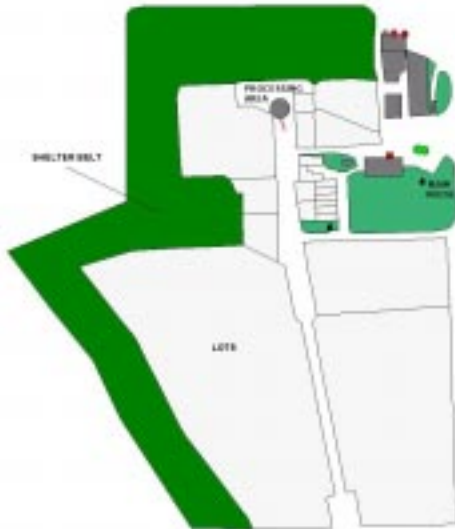
After using the Leica GS50 GPS/GIS unit to capture GPS data on the feedlot, Planning District III created GIS maps showing the location of feedlot facilities.
