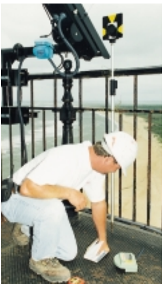
Leica prisms were mounted on the top and the base of the lighthouse and checked every day. The black box is the housing for the Internet site camera.
