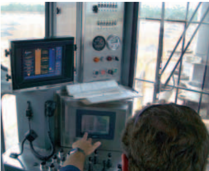
With DrillNav Plus, mines can design drill patterns in the office and download them to the drill where the operator follows the coordinate of each hole to be drilled
