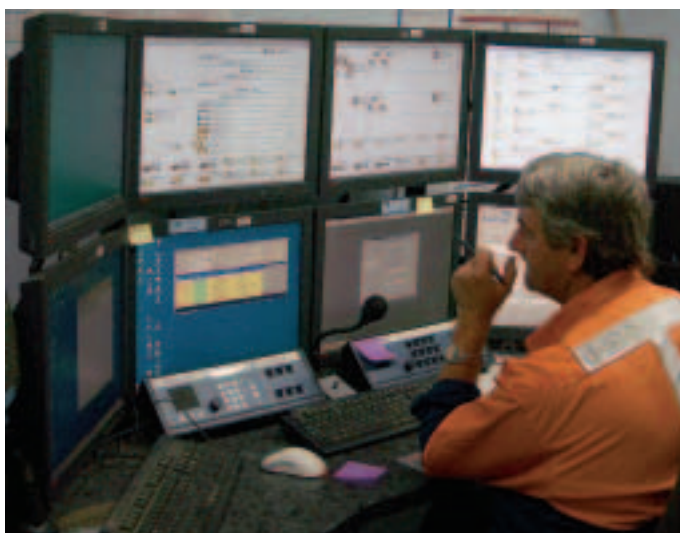
(Below): A Dispatcher using the GPS-based FMS system to locate and report on any of the machines on the mine
