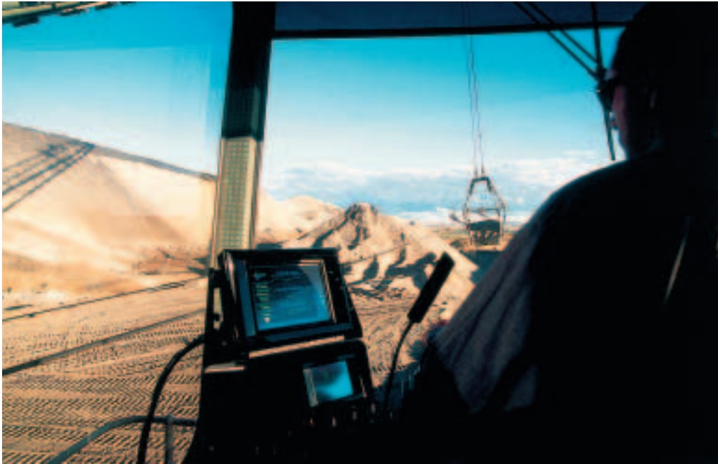
(Above): An Operator receiving real time feedback from the Series 3 9000 Dragline monitor
