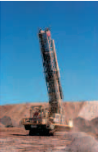
With DrillNav Plus, mines can design drill patterns in the office and download them to the drill where the operator follows the coordinate of each hole to be drilled
