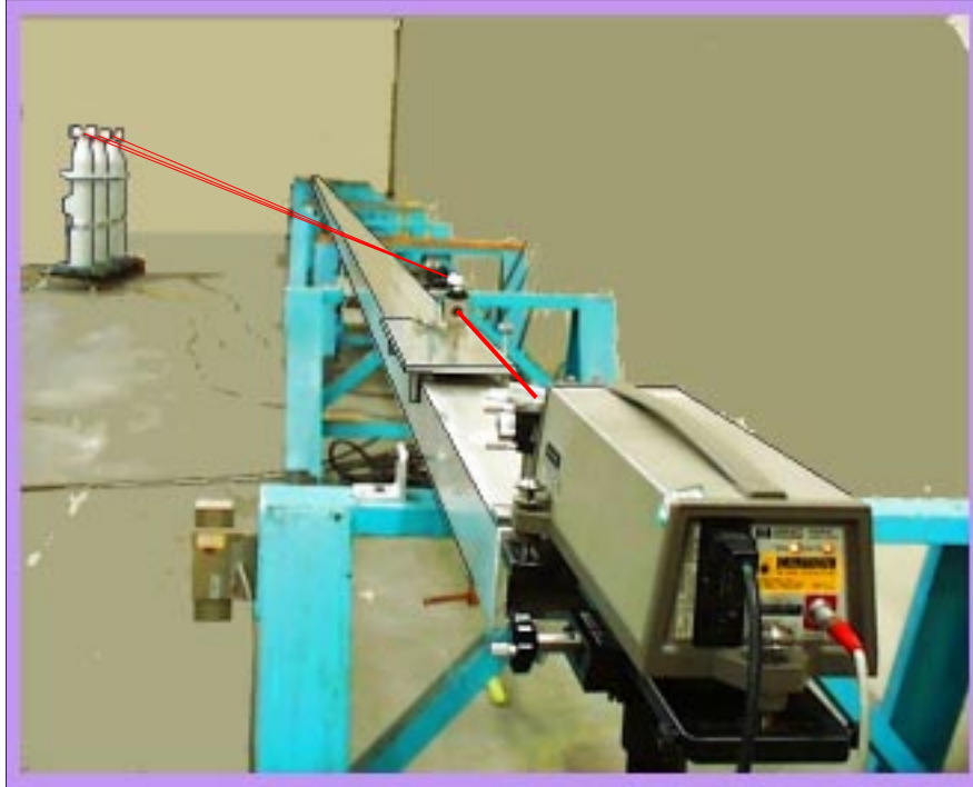
Figure 5: Lateral test setup of three laser tracking interferometers with the reference linear interferometer in the foreground.
