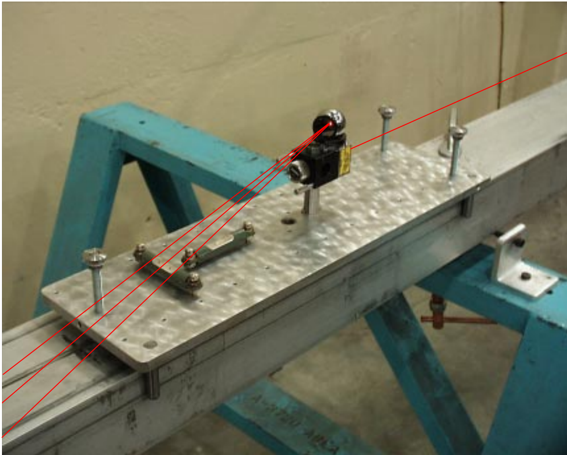
Figure 3: Target sled setup for lateral test. (Lines-of-sight for three tracking interferometers and the reference interferometer have been added.)
